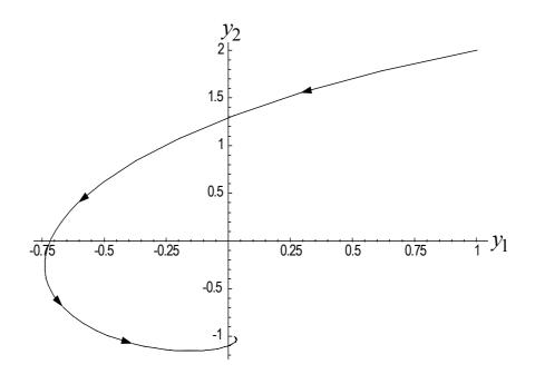
If the root has a real part closer to zero we get more pronounced circles. Here is a phase diagram with a real part of -0.1.
