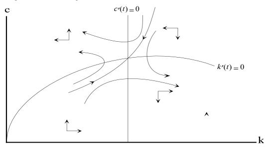
We conclude that this system has saddle point characteristics and thus have only one stable trajectory towards the steady state.
